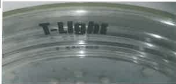
Manufacturer's trade name and required symbols for the stop/position light and the rear direction - indicator light
