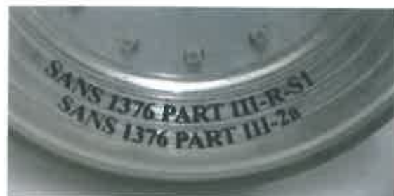
Manufacturer's trade name and required symbols for the stop/position light and the rear direction - indicator light
